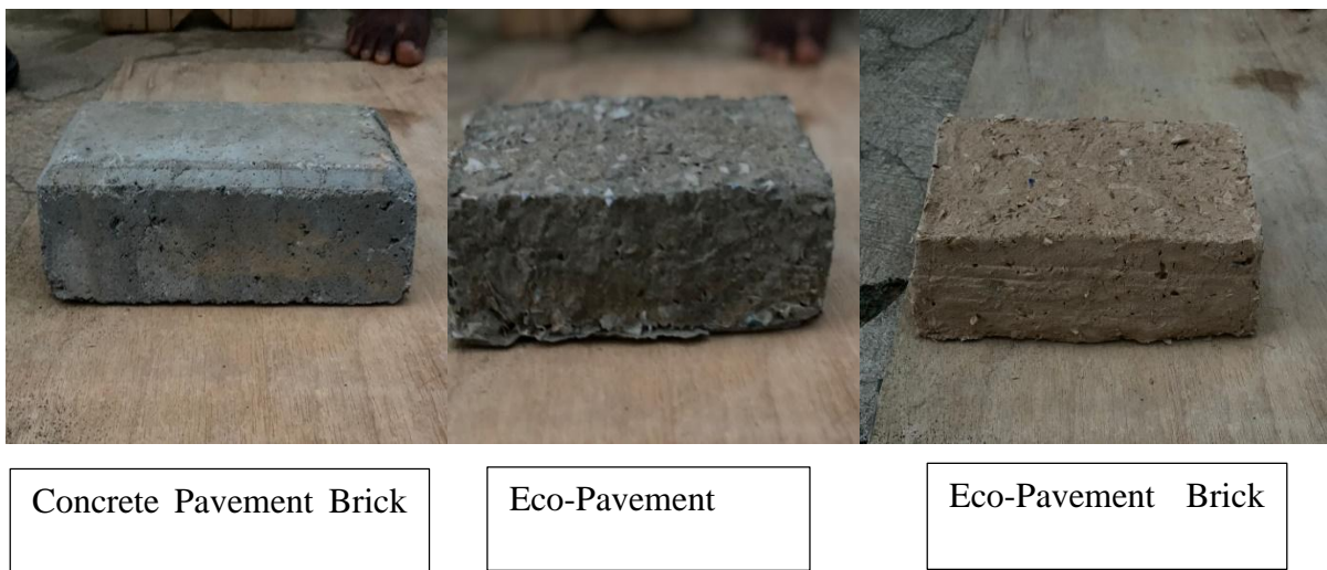
Figure 3: Constructed eco-pavement bricks and an acquired concrete brick.
